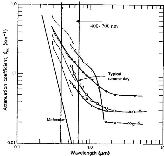
Fig. 3. Attenuation coefficient versus wavelength for a 16.25 km path at sea level (Yates and Taylor, 1960 and McCartney, 1976).
