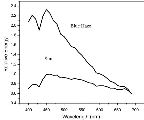
Fig. 6. The relative energy of the D6500 “sun” compared to “blue haze.”
