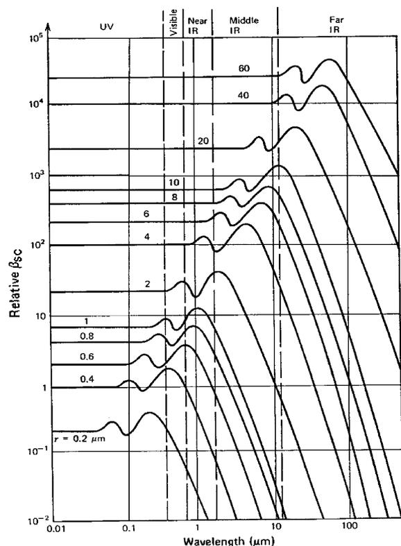
Fig. 2. Relative values of total scattering coefficients for different wavelengths and various particle radii (from Gaertner, 1947 and McCartney, 1976).
