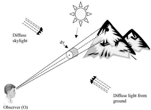
Fig. 4. Source of the air light between an observer and an object, and apparent luminance of an object due to the airlight (after, Middleton, 1952, derived from McCartney, 1976).
