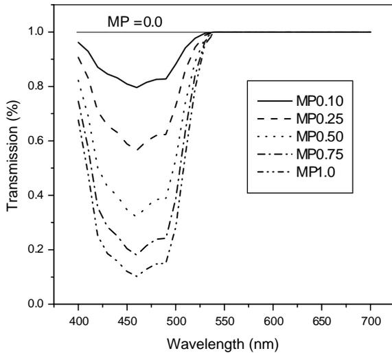
Fig. 7. The percentage transmission versus wavelength corresponding to MP absorption with peak absorption values ranging from 0.0 to 1.0.
