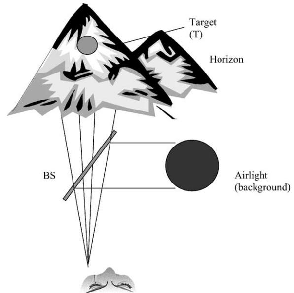
Fig. 5. The observer at  $O$  views the target,  $T$ , along a haze aerosol path. The light scattered into the eye, the air light, from the same path is considered separately and is symbolically represented as if being reflected by a beam splitter,  $BS$ .
