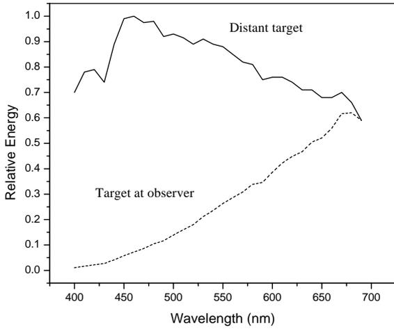
Fig. 11. Solid curve shows the spectral energy of a D6,500 illuminant that is reflected from a spectrally flat target; the dashed curve shows the spectral energy of this same light after it has passed through the intervening atmosphere where  $\beta = c\lambda^{-2.0}$ .
