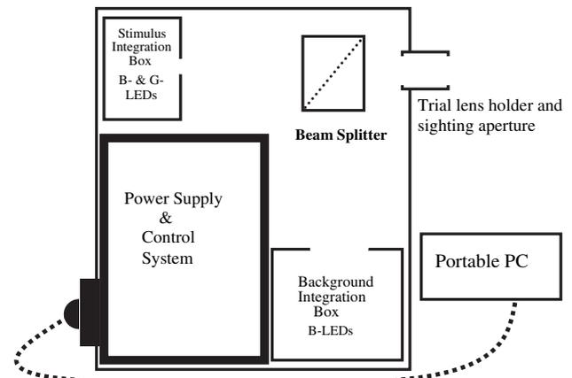
**Figure 1.** Design layout of the measuring device.
